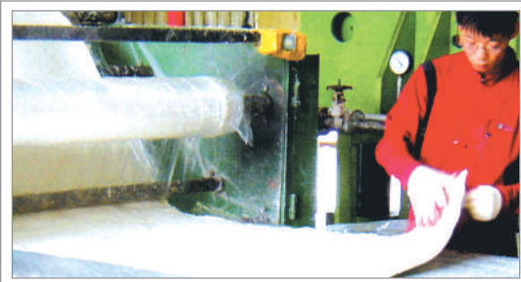
02 GRP Raw Material Cutting
